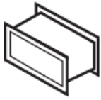
Pre-chamber anti-flow device without inlet flange Maximum operating pressure 0.5 bar
